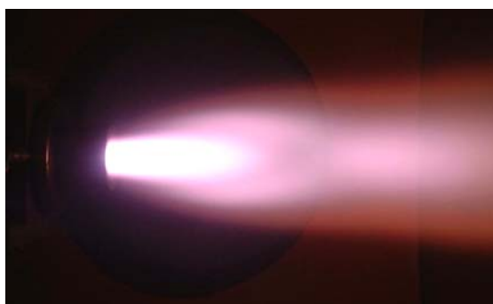
Fig. 4: Photograph of a free argon plasma jet (60 A, 44 V, 30 Pa background pressure). The jet structure and boundary are clearly visible. The dark zone at the jet centre corresponds to the zone of silence; it is located just ahead of the normal stationary shock wave. The red colour visible at the jet boundary is a sign for air drag (continuous release of a minute amount of air in the vessel).
